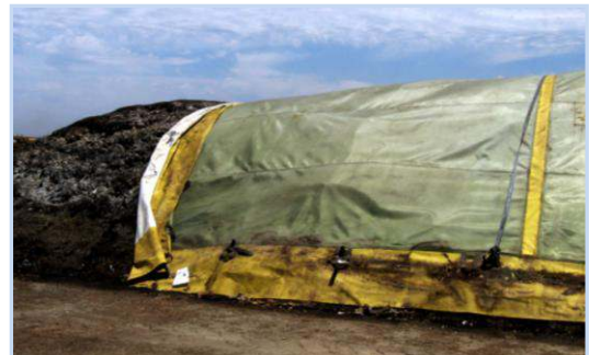
Exhibit 9: Aerated Static Pile System
